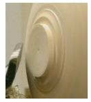
Now dovetail the chucking point, making the base around it slightly concave, which will help in centring the work on the chuck. It is important to get the diameter of the chucking point as close as possible to the optimum diameter of the chuck (that is, where the jaws form a perfect circle) – this will also help to centre the work on the chuck and will also reduce the amount of marking the jaws make on the wood.
