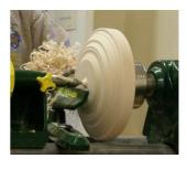
help the tool drift you can put a bit of liquid paraffin on the back of the chisel.
